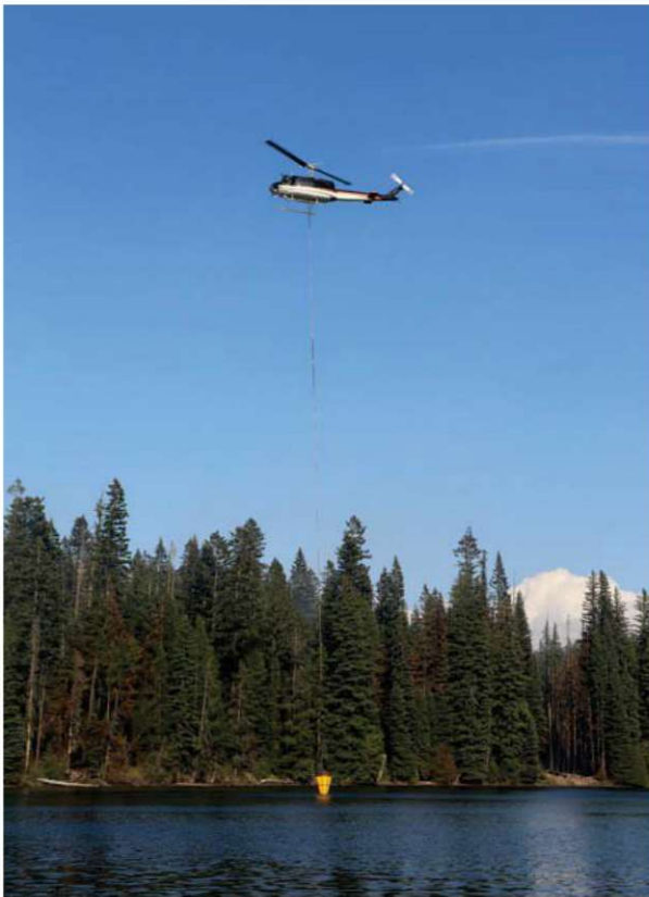
FIGURE 21-5 Rotary-wing aircraft can be used to apply water to a wildland fire by either A , carrying the water in an internal tank and dropping it directly on the fire, or B , by using a long cable and bucket system to transport the water to the scene.
